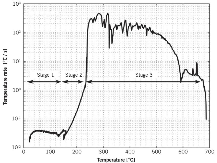
FIGURE 1 Temperature curve, from phase 2 thermal runaway (© Hugo Benzing)
